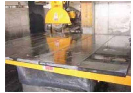
Bridge Saw Use continuous diamond porcelain cutting wheel.
