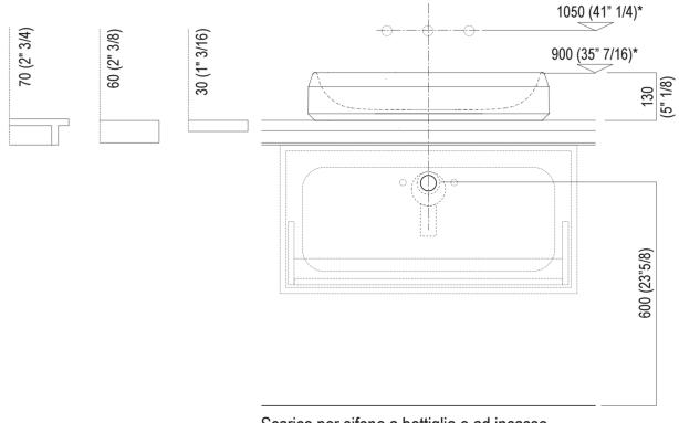
Scarico per sifone a bottiglia e ad incasso Drain for bottle trap and concealed waste trap
